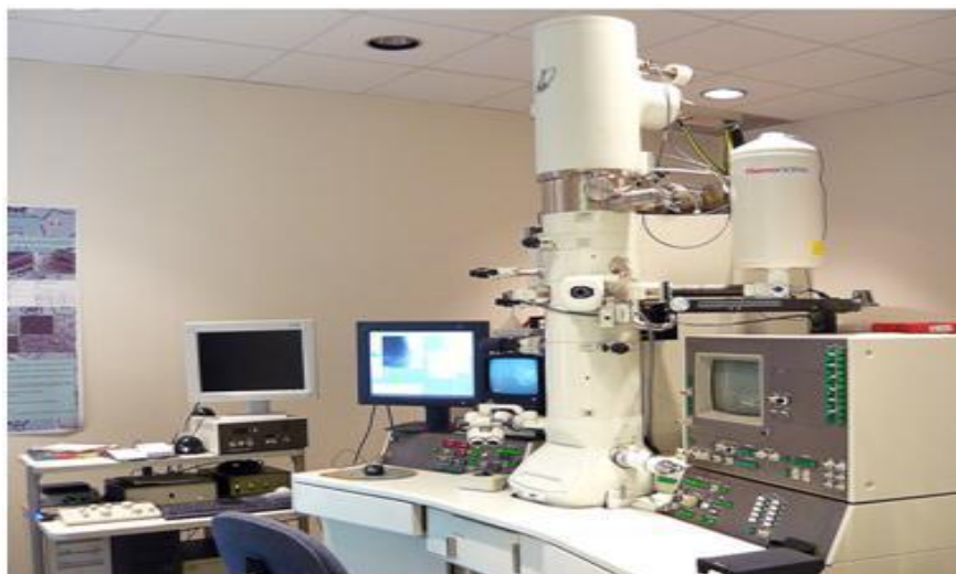
Figure 43: Transmission electron microscope (TEM) JEOL JEM-2010F , physics institute, UNAM.
