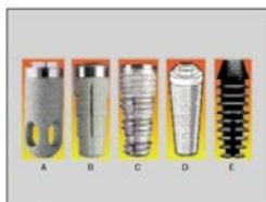
Fig 14 Press-fit body geometry variations, consisting of straight cylinder (A), tapered cylinder with steps (B), threads (C), or straight wall configuration (D), and a finned taper design (E).
