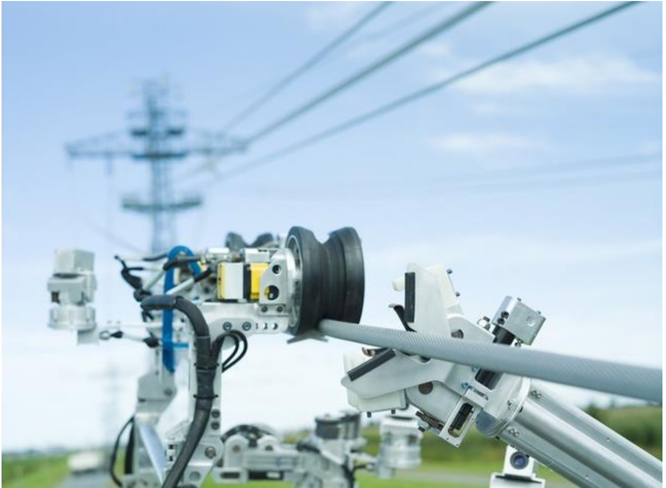
Figure 1.8 – Device Line Scout on overhead line
